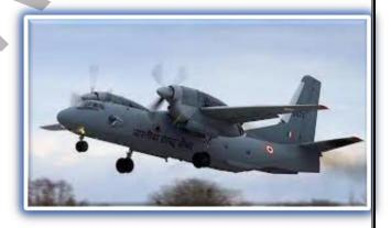
As part of efforts to lessen its carbon footprint, the Indian Air Force (IAF) is seeking to fly an AN-32 transport aircraft modified to fly 200 combat hours on 10% blended biodiesel within the next six months, according to Air Vice Marshal S.
