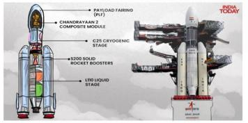
The LVM-3 is a heavy-lift launch vehicle, which means that it can carry a large payload into space. It is the most powerful rocket that ISRO has ever developed, and it is unmatched in its class. Christened as the 'Bahubali' of rockets, LVM-3 is a three-stage rocket, consisting of two solid-fuel boosters and a liquid-fuel core stage powering it. The solid-fuel boosters provide the initial thrust, while the liquid-fuel core stage provides the sustained thrust to
